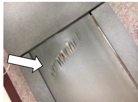
Worn Walking Belts with Separating Seams
